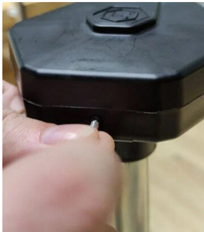
Fig.104 Extracting the seal
