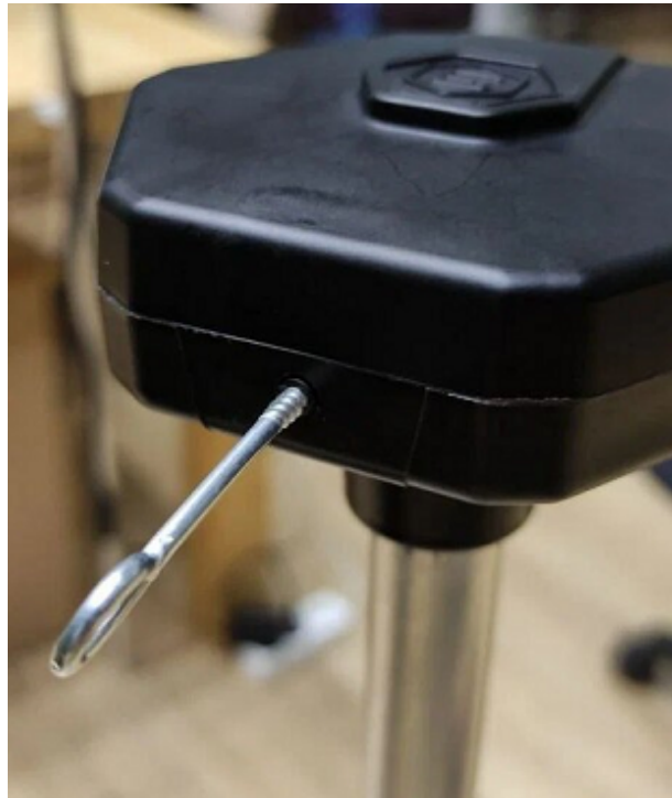
Fig.103 Key screwed in the seal
