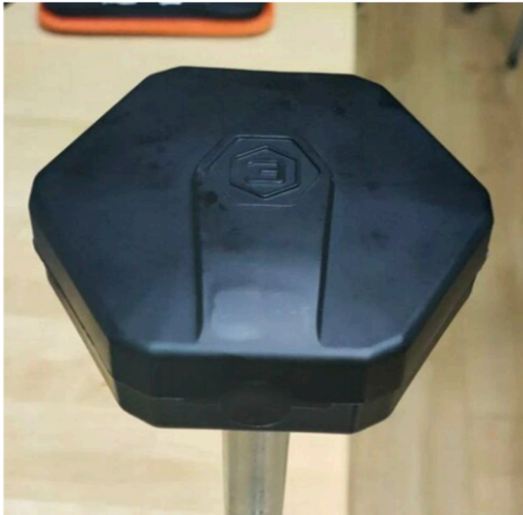
Fig.101 Sensor with protecting cap on it
