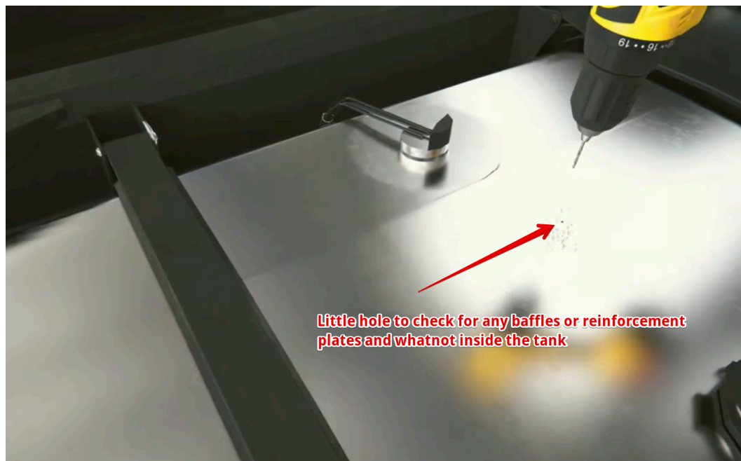
Fig. 29 Drilling a hole to later probe for any obstacles inside with a piece of wire
