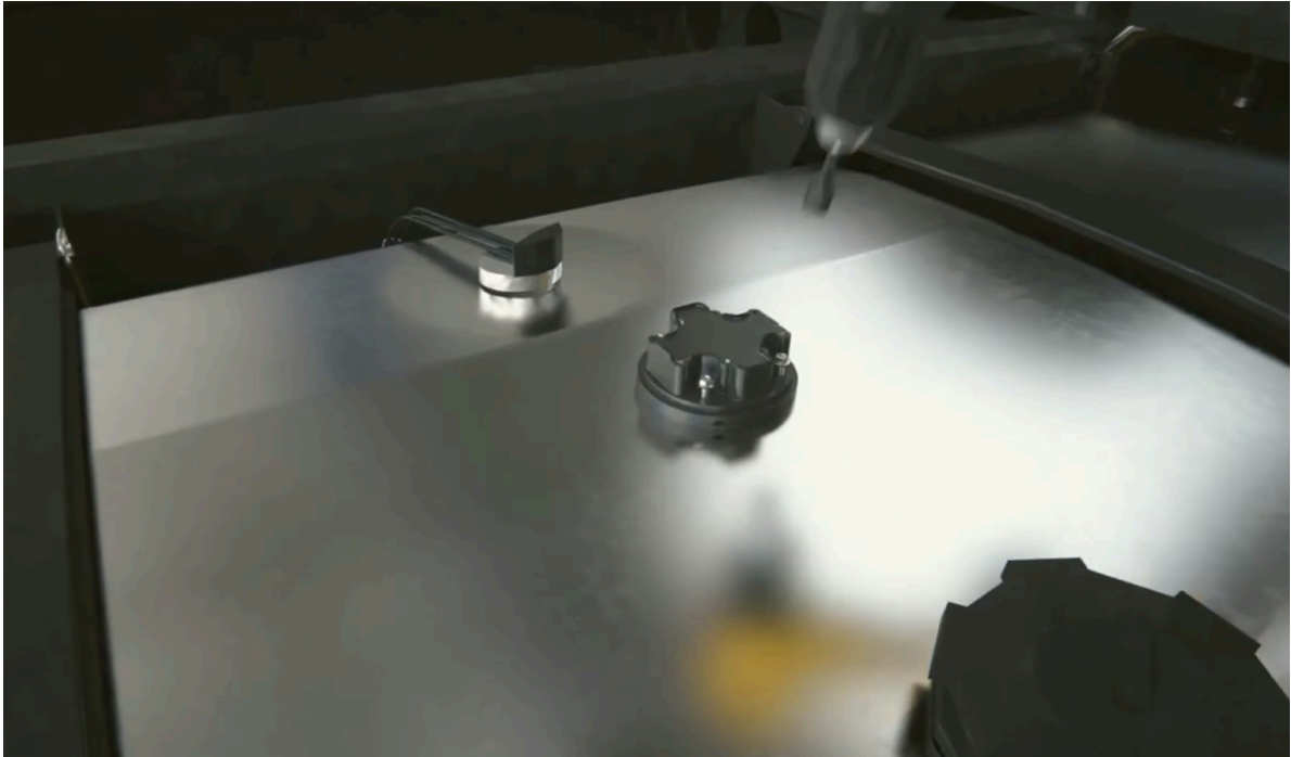
Fig. 42 Fixing the self-tapping screws
