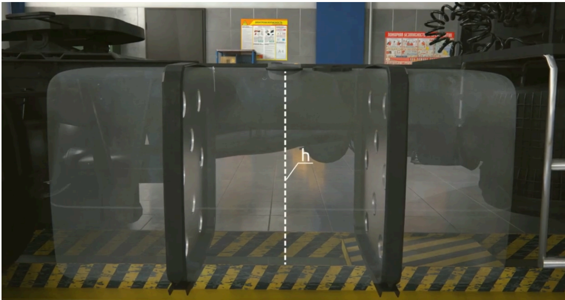
Fig. 33 Measuring the height of the tank
