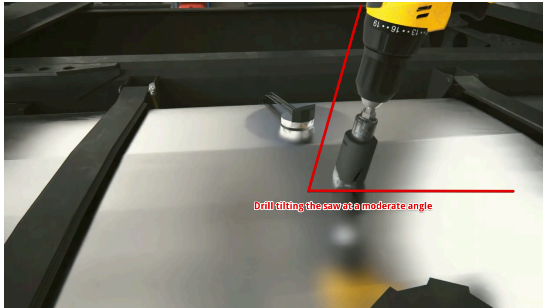
Fig. 30 Drilling a hole at an angle
