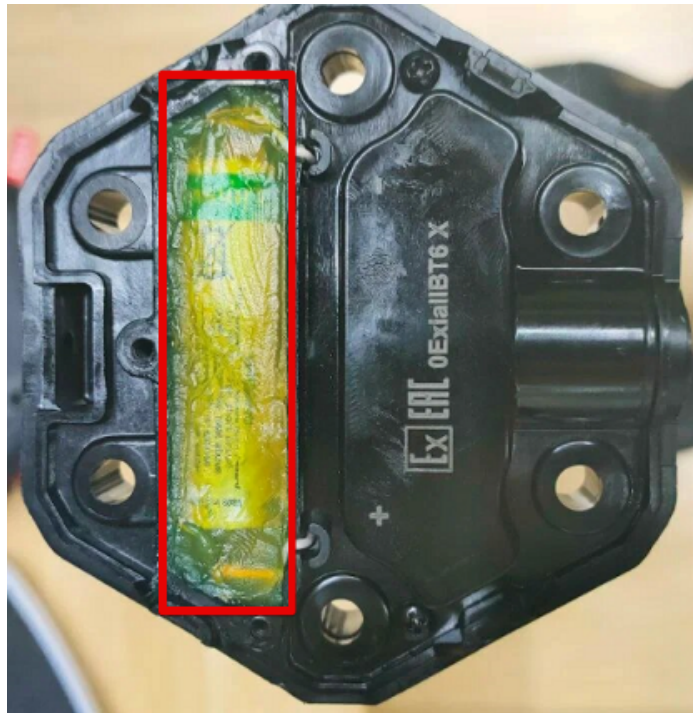
The battery holder's cavity filled with the litol
