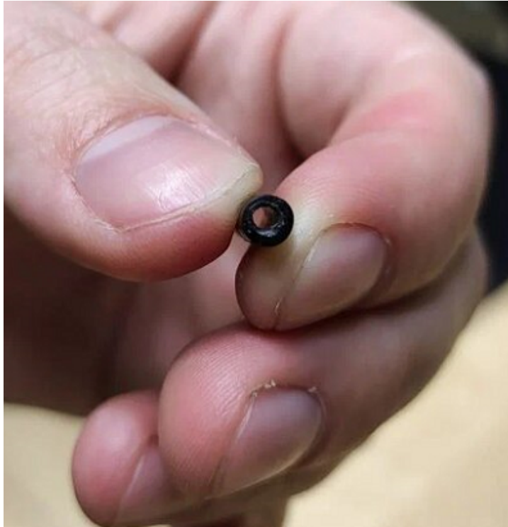
Fig.105 Seal after extracting (its covered end is damaged)
