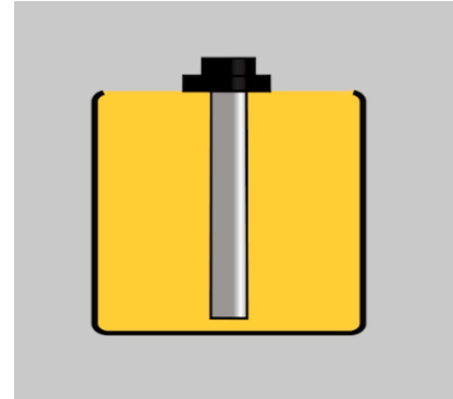
Fig. 18 Filling the tubes by putting the sensor into fuel
