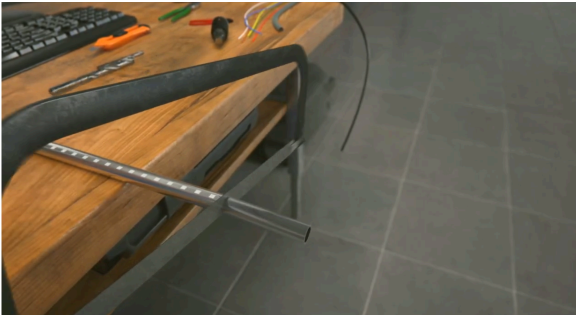
Fig. 35 Cutting the tubes
